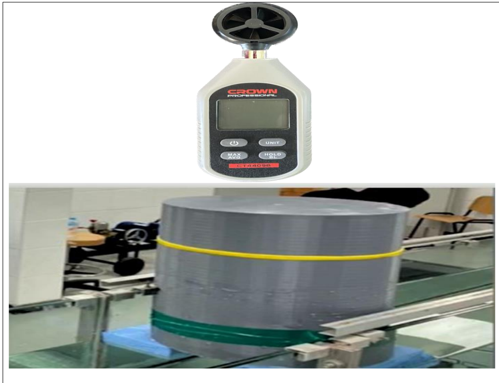
Figure 5 The air chamber model and the anemometer
