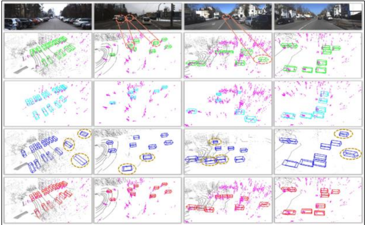
Figure 6 The qualitative results produced by the M2-Fusion model using the Astyx HiRes 2019 dataset. The first row displays RGB images of the driving scenes. The second row shows the ground truth annotations, where green bounding boxes highlighted by dotted orange ovals indicate missed detections. The third row illustrates object detection results using radar data alone, while the fourth row shows results using lidar only. In the lidar results, blue bounding boxes surrounded by dotted brown ovals represent false positives. Finally, the last row demonstrates the outputs of the M2-Fusion approach, where the fusion of radar and lidar data leads to more accurate detections by reducing both missed detections and false positives
