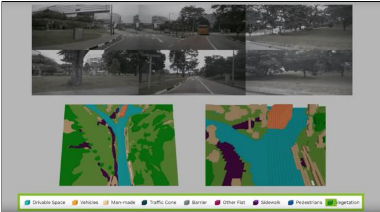
Figure 5 NVIDIA wins the 3D Occupancy Prediction Challenge with FB-OCC, a technology designed for using camera data to generate 3D voxel bird's-eye maps. The bottom two maps exemplify the creation of voxel grids using sensor data from the six camera inputs above [23]
